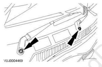
2. Remove the wiper arm nuts.
